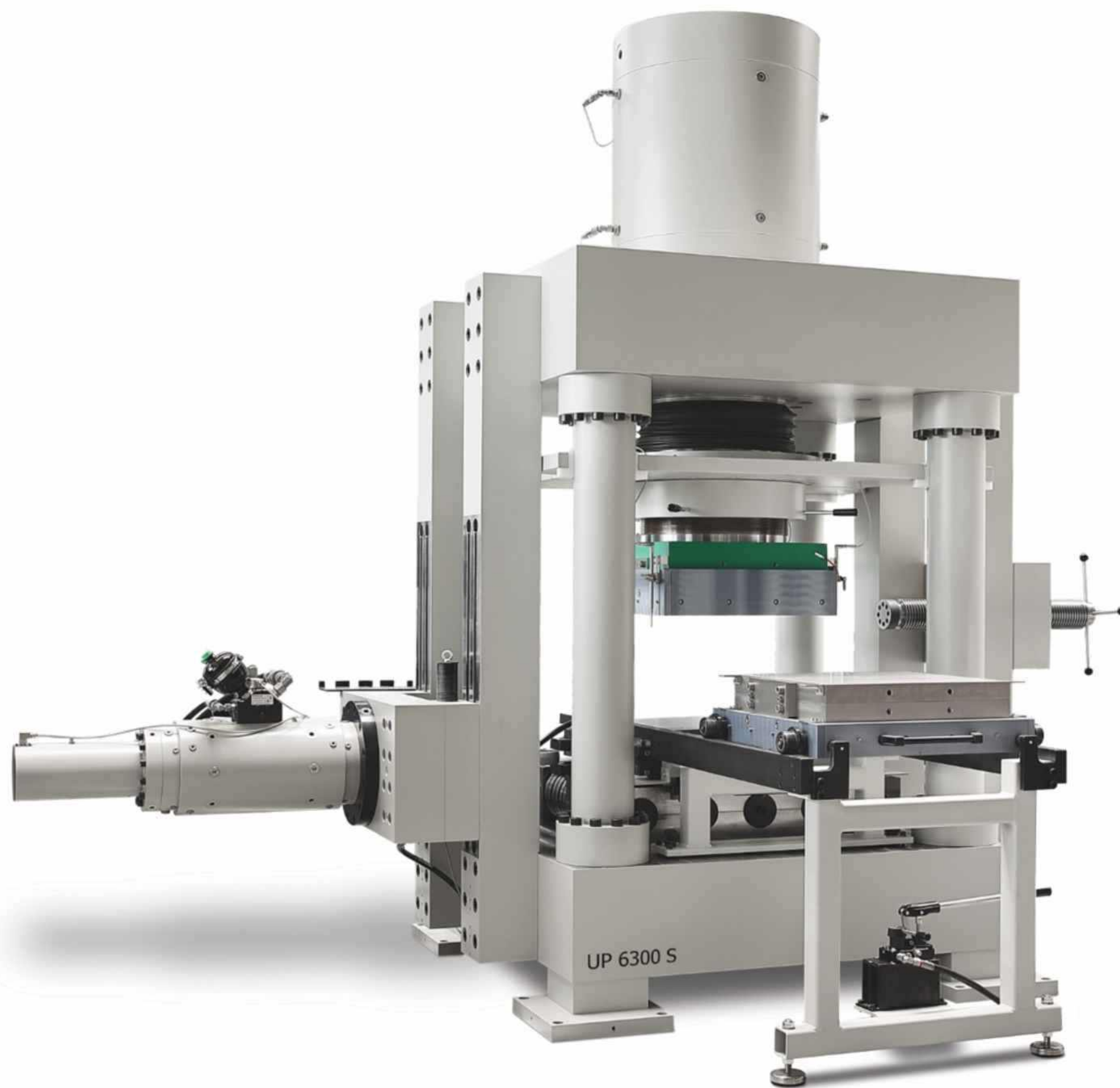
Schematic Diagram of Shear Modulus Test Equipment Compression-Shear Testing Machine (Double-Shear Configuration) acc. EN 1337-3
