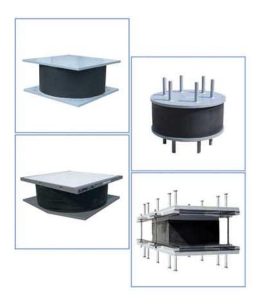
Mechanical forces including horizontal, vertical loads and rotation around different axis (torque) and simultaneous deflection pressedon a structure combine with tensions caused by structure's materials expansion and contraction, temperature, creep and complicated movements. To prevent and control these movements elastomeric bearings are used.
